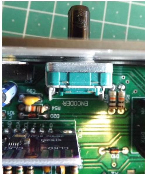
**Do not screw the Encoder. This is sufficiently attached to the EGV-9B PCB.**
