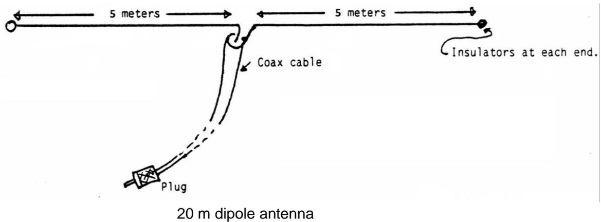
For the antenna "arms" you can use any cable strong enough to hold the weight of the coaxial cable hanging. Install the antenna in the highest and clearest position possible.
