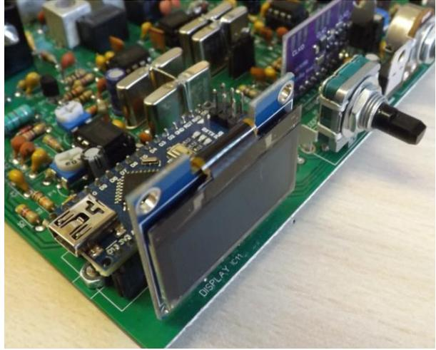
You may prefer to install the OLED display, encoder and potentiometers outside the board. Then see the section "WIRING AND CONNECTIONS"
