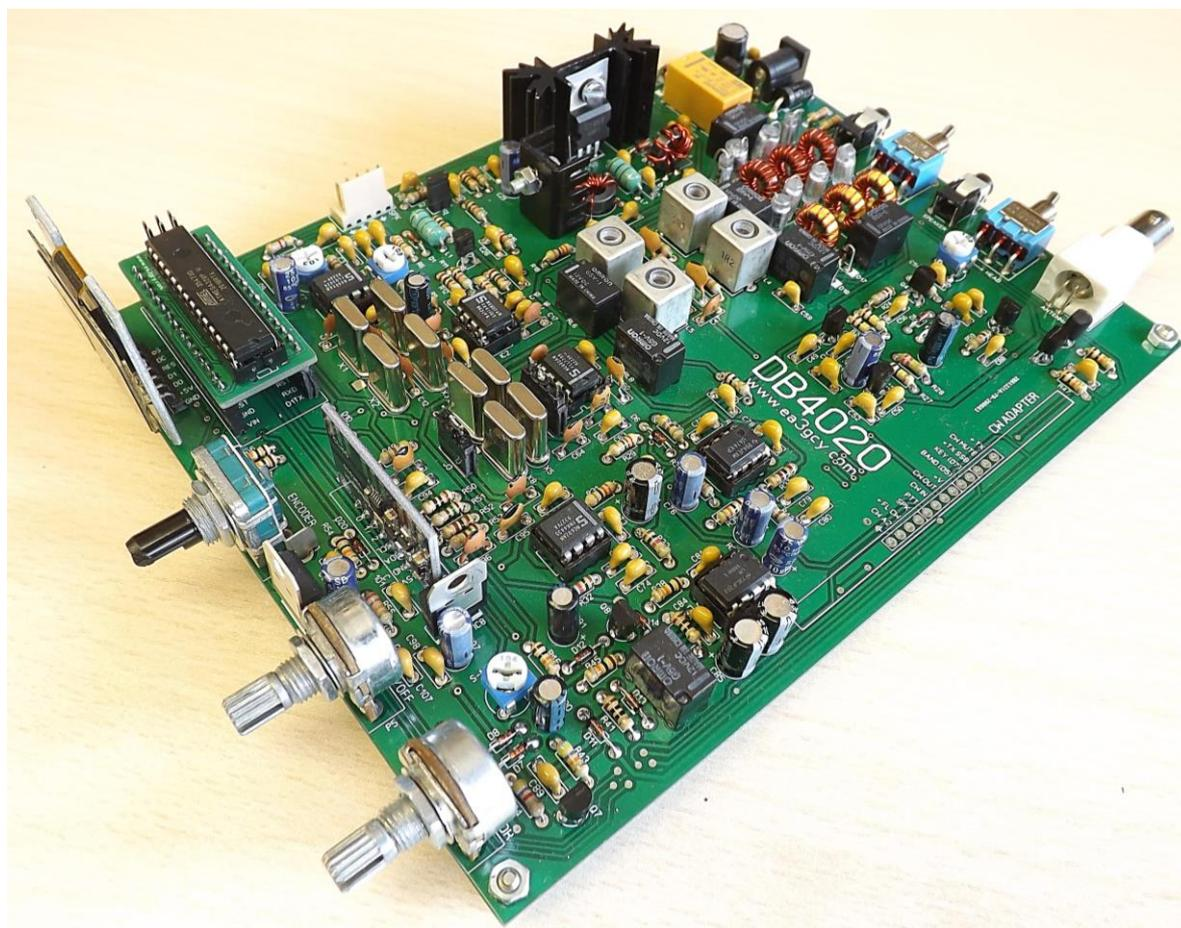
Thank you for building the **DB4020** Dual Band 40&20M SSB Transceiver kit
