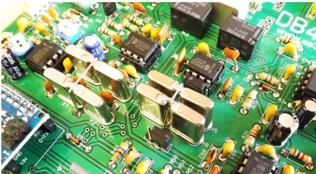
*Note: With a scrap piece of wire left, you can solder the crystals housings to GND.*
