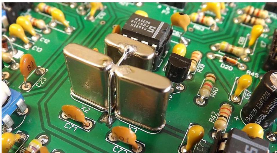
Note: *With a scrap piece of wire left, you can solder the crystals housings to GND. Be careful not to overheat the crystals.*
