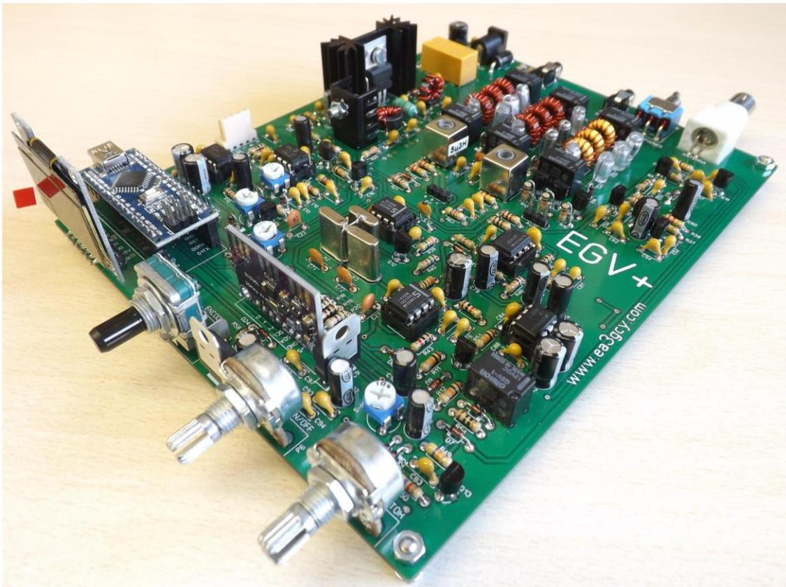
Thank you for building the **EGV+v2** 40, 30 and 20m QRP CW Transceiver kit
