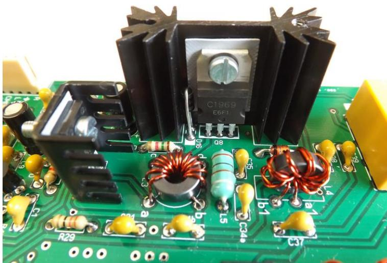
If you plan to work at maximum power and for long periods of time (at base station) it may be advisable to increase the cooling surface. You can add some system to increase the temperature dissipation, for example by an auxiliary metal surface, a mini-fan or other similar system.
