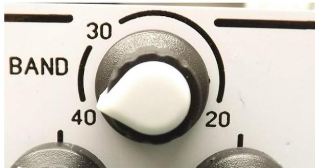
With an antenna connected to the transceiver tune to any frequency in the 40m. Alternately adjust L1 and L2 until obtaining the maximum noise level in the speaker. Now, try to tune in a stable signal within the band and readjust L1 and L2 alternately until you hear it at the highest possible level.
