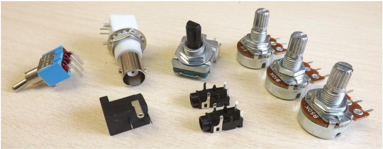
Before mounting the external connection jacks, you should cut the protrusions located at the bottom of these jacks; otherwise you will not be able to solder them in the correct position. See the image.
