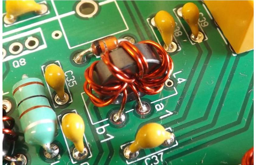
Note: For greater clarity, the drawing shows one black wire and one red wire. In reality, both wires are of the same color. You can mark the "a" -"a1" with a marker pen.
