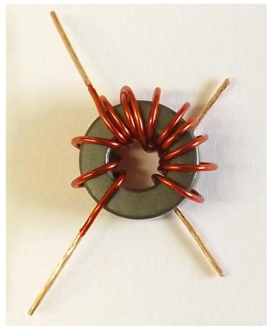
IMPORTANT: Wind the toroid exactly as shown in the images. You must pay attention to number of turns as well as to the direction of the winding.
