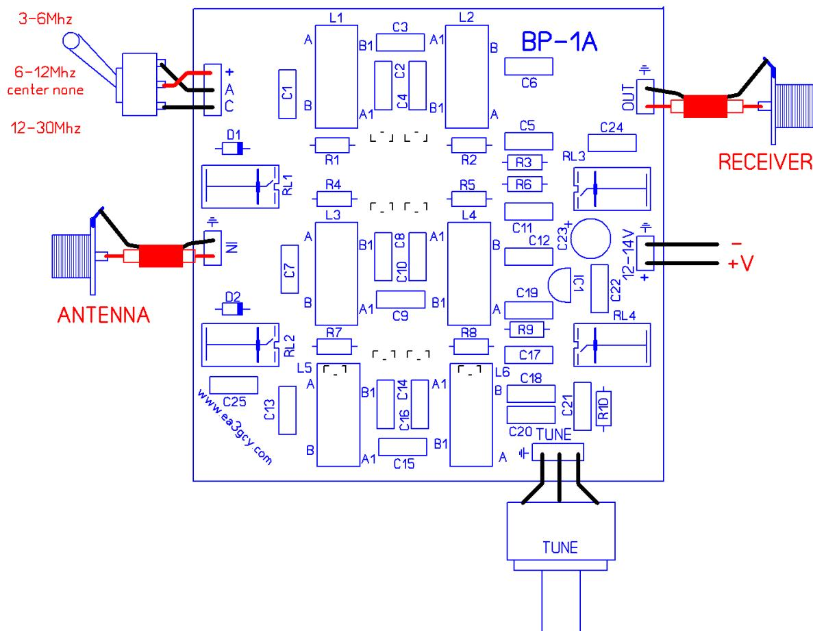
The antenna input is marked "IN" and the output to the receiver is marked "OUT" (use 50ohms coaxial cable for both connections)
