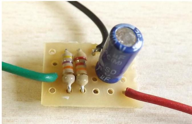
You can mount the resistors and the capacitor on a small perforated board or you can mount the components "in the air" directly on top of the ILER board.
