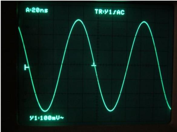
10 MHz output signal. Perfect sinusoidal form.
