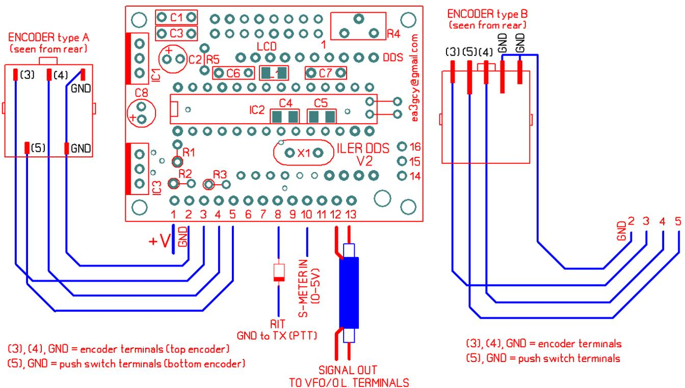
The wiring described is from the back of both the encoder and the control board.
