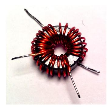
As with T1, cut the pigtails to fit the pads and solder them to their correct pads "a" –"a1" and "b" – "b1". Be sure of their correct orientation. This toroid may be left touching the board or slighlty separated, 1-3 mm (1/16 in) over the board.
