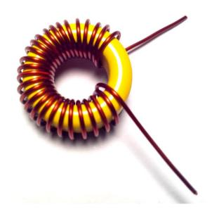
Make tight turns, following the contour of the toroid so turns are taut. Spread the turns over the toroid and leave 10 mm (0,4 in) pigtails. Scratch and remove the enamel so the pigtails may be soldered. Turn counting: every time that the wire goes through the inner hole of the toroid it counts as one turn.
