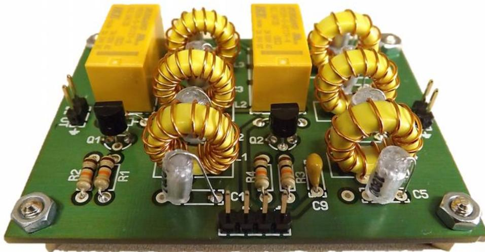
Thanks for constructing the **LPF-4B** low pass filter kit
